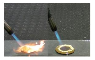
The most widely used nonhalogenated replacement for flame retardant in the world due to its versatility and low cost is alumina trihydrate (ATH). ATH is non-toxic, halogen-free, chemically inert, and has low abrasiveness. Further, as it is available in different particle sizes, it can be used in a wide range of polymers at processing temperatures below 220°C. When an ATH-filled composite is subjected to temperatures above 230C/446F,
